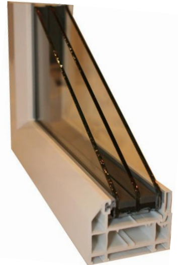
Cross section of 2500 Sculpted frame 40mm triple glazed unit and 3038 bead
