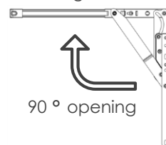
Acts as an easy clean and fire egress hinge as it pivots and opens 90 ° like a traditional butt hinged window.
