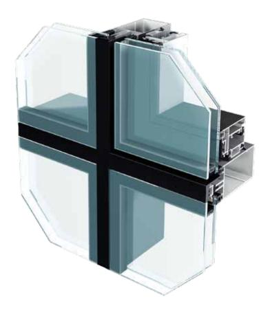
Elegance SX IT is an opening window developed for use within curtain wall facades whereby the opening light frame is not visible externally. Elegance SX IT allows the external glass surface to be positioned precisely in line with that of the adjacent fixed curtain wall areas, when combined with the absence of an external frame this means that the opening windows are virtually indistiguishable within the overall facade grid.
