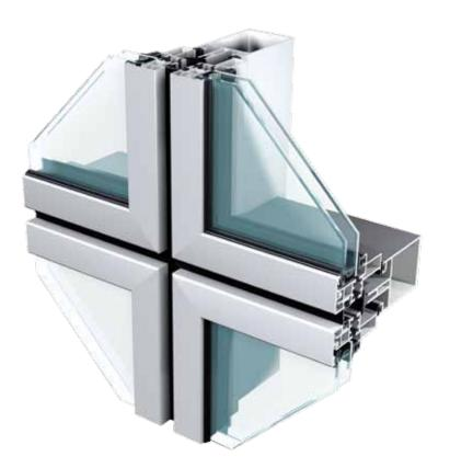
Elegance 52 GF is a curtain wall system based on the structure of the Elegance 52 SG using a glazing bead instead of structurally bonding the glass to the panel. Our design team developed this solution to offer a version where the glass is held in position with aluminium as in a picture frame. This approach offers each panel to be independent but still be integrated in the full curtain wall.
